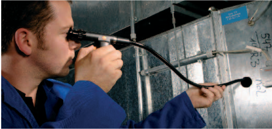
Checking in an air conditioning duct with gooseneck covering, medium flexibility.
