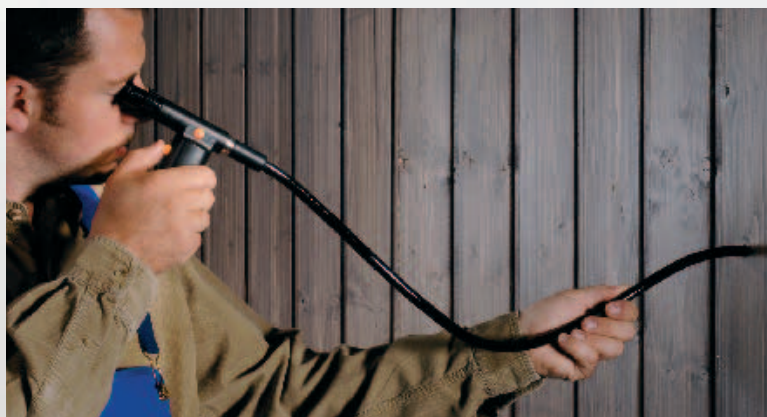
Checking insulation using the inherent stability of the decabon tube
